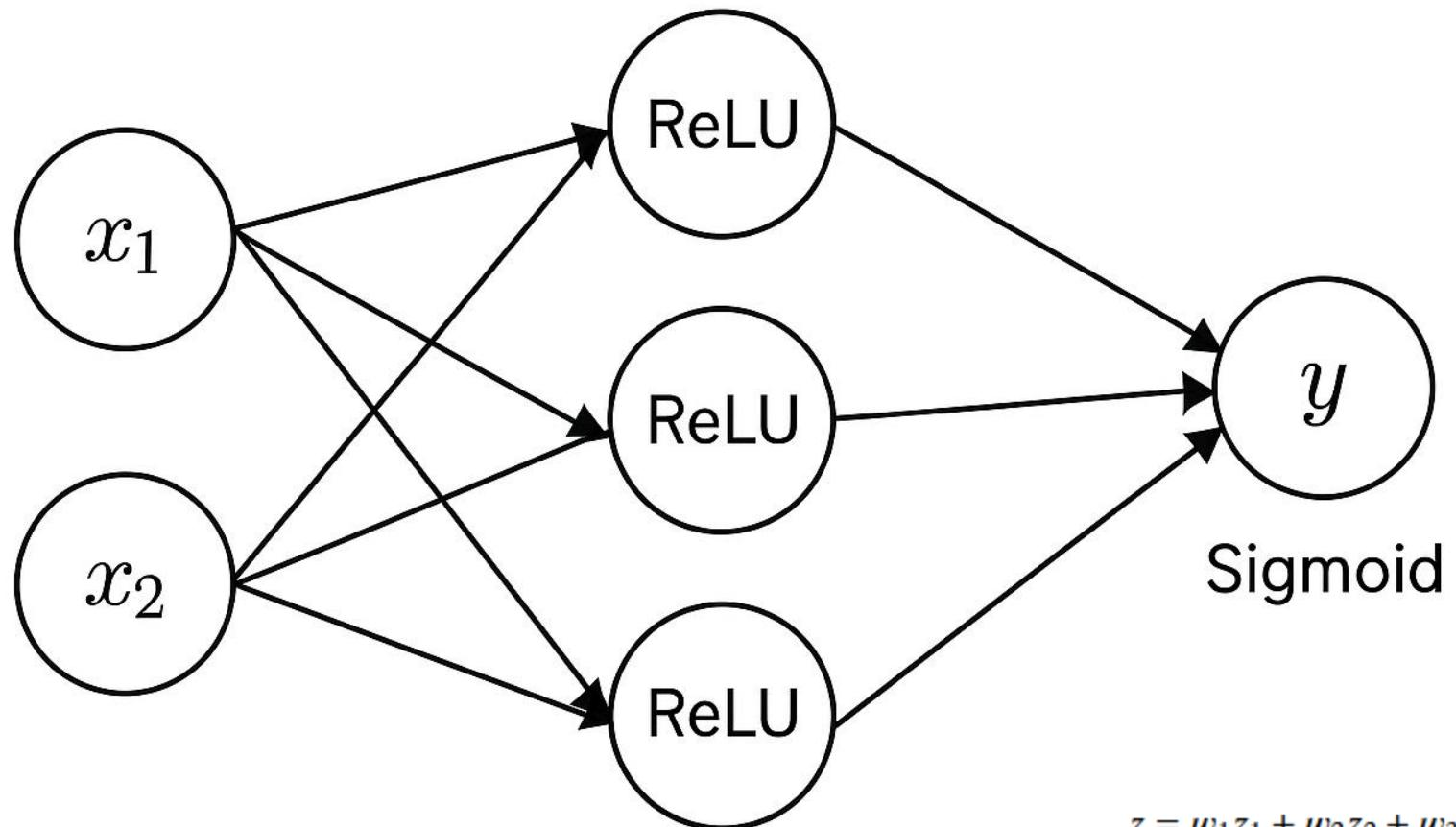
$$z_1 = \max\{0, (x_1 * v_{11}) + (x_2 * v_{12}) + b_1\}$$
